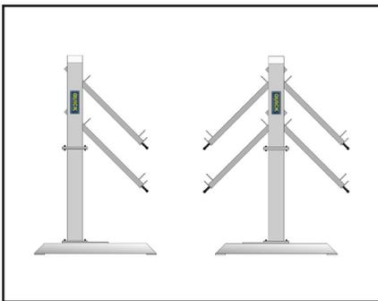
The innovative "two-sided" frame design allows for either one-sided or two-sided operation, at the shop owner's discretion. The one-sided configuration allows for placement of the frame tightly against a wall, for maximum compactness. The two-sided configuration doubles the amount of easily-accessible clamping area, for industry-leading "room to work." The Rack is configured by choosing either of the two available foot mounting positions.
