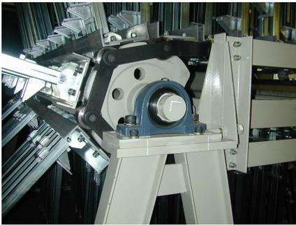
QUICK High Production Clamp Carriers are available in widths (maximum stock length capacities) of 6.5', 8.5' (standard), 10.5', 12.5' or 16.5', and 20, 30, 40, 60 or 80 sections. Machines can be outfitted with either one or two sets of Clamp Tighteners (Pneumatic or Hydraulic) and Panel Flatteners. A 20-Section Carrier can be expanded to 30 sections at a later date, and a 30-Section Carrier can be expanded to 40 sections, if desired.
