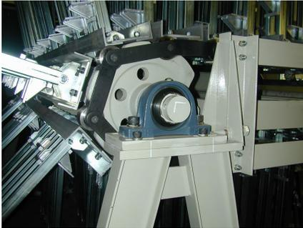
the industry, featuring oversize frame rails and runways, massive 3" diameter front and rear shafts (large-diameter shafts resist twisting when the Carrier is being indexed from section to section by the drive motor; 3" shafts are 4 times stiffer and stronger than 2" diameter shafts), big cast iron sprockets, heavy-duty chains with 2" wide rollers, and extra-stout 6" I-beam legs. Machines are available to handle stock up to 20.5' long and 8" thick. Frames are expandable to up to 80 sections.
