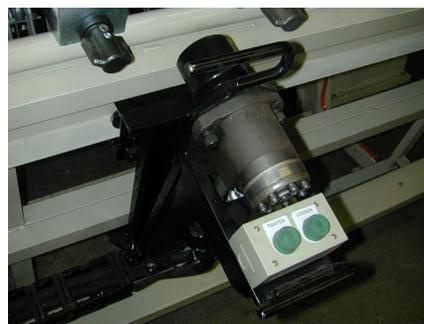
clamp screws eliminate the need for manual rear jaw adjustment. All adjustment is made quickly by the Clamp Tightener itself.
