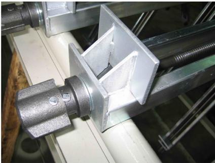
rosion-resistant, zinc-plated steel clamps with full box frame construction and 3/4" diameter full-length screws. The clamp jaws are 2-1/2" high, and angled inward one degree to keep stock held down securely in the clamps. Rocker Plates for face gluing are available. Standard clamp opening is 38"; other lengths are also available.
